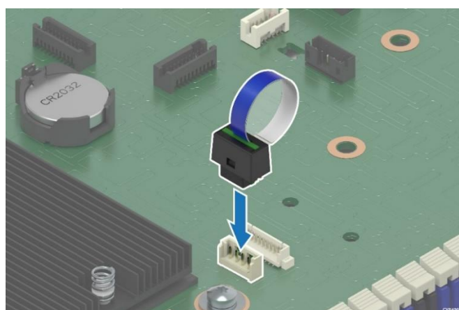
Figure 175. Intel® VROC Key Insertion
