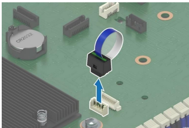
Figure 174. Intel® VROC Key Removal
