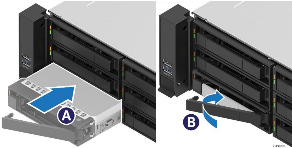
Figure 149. 3.5" drive Assembly Installation
