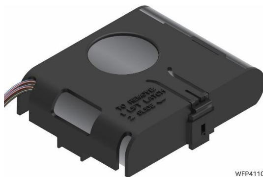
Figure 79. Insert Super Cap Battery
