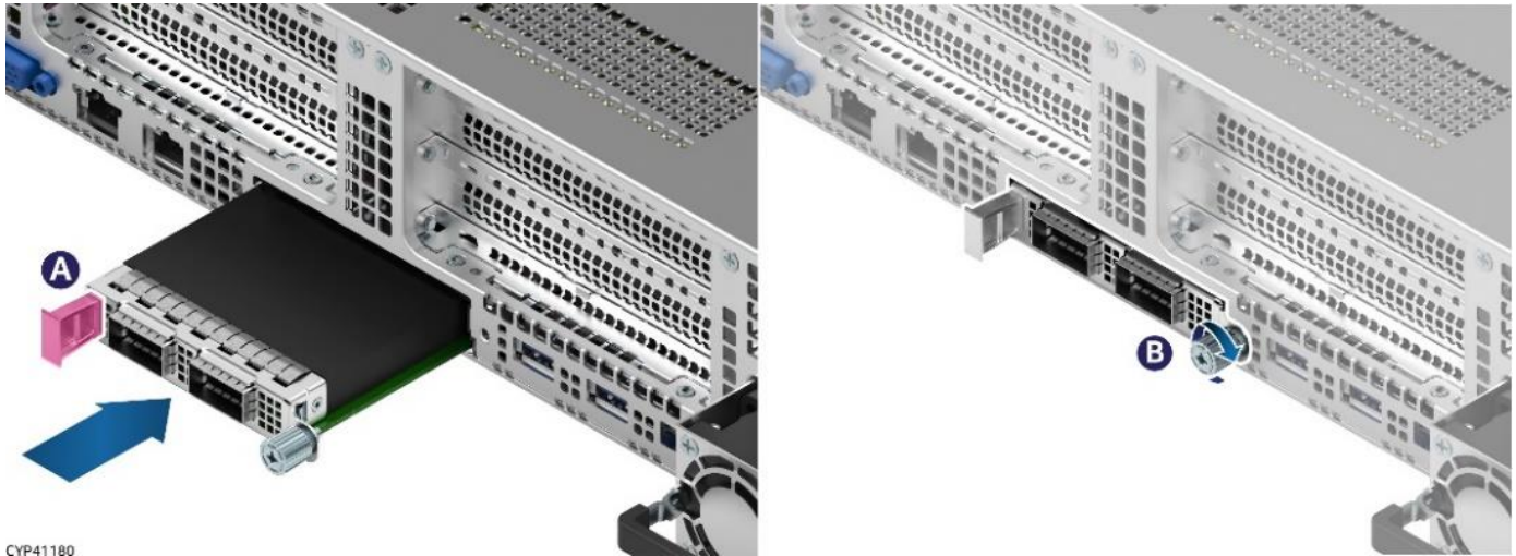
Figure 62. OCP* Adapter with Pull Tab Installation
