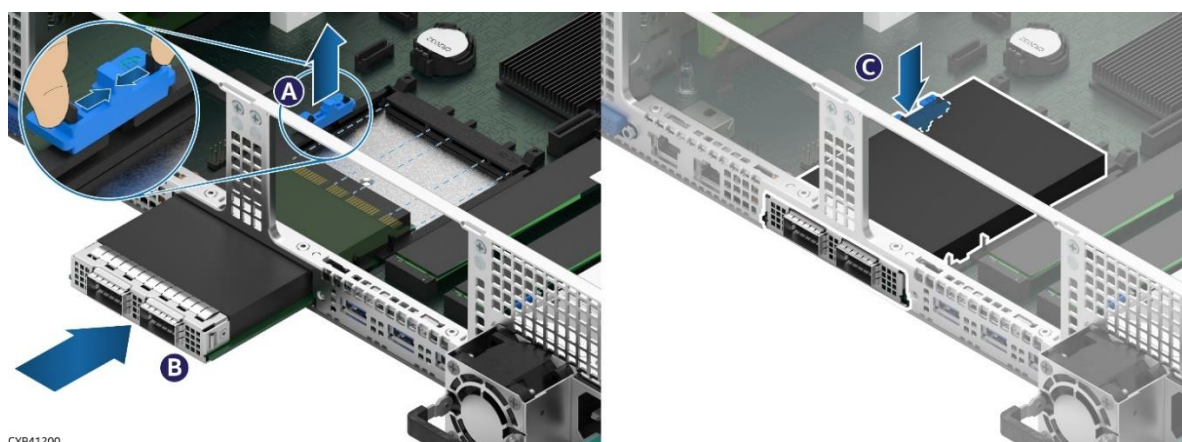
Figure 65. OCP* Adapter with Internal Lock Installation
