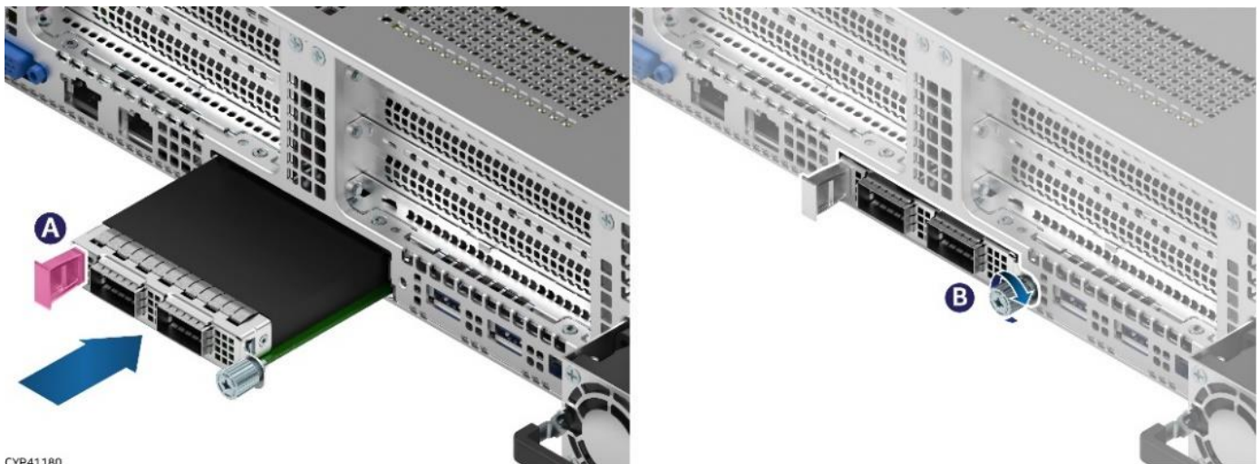
Figure 156. OCP* Adapter with Pull Tab Installation
