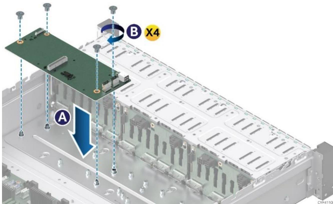
Figure 75. SAS Interposer Card Installation
